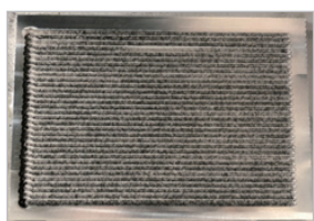
7N01 铝基样品实物扫描图 (200mm*160mm)
